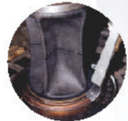
Clean every part of the mold including the bead ring.
