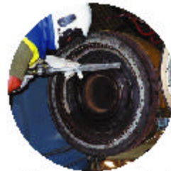
Molds can be cleaned while they are hot and in the press.
